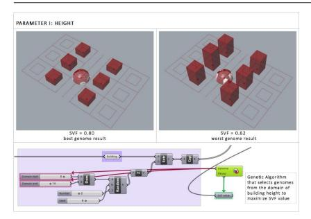
Figure 8. The SVF simulation based on the parameter, *building height*
