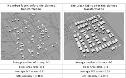
geometry on the condition of heat island intensity in the built fabrics.
