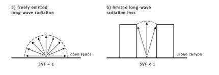
Figure 1. The relation between SVF values and emitted long-wave radiation
