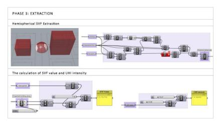
**Figure 7.** Phase 3: Extraction of the SVF from the hemispherical projection model
