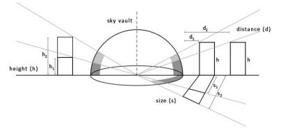
**Figure 3.** Schematic illustration of the effect of major parameters on the visibility of the sky
