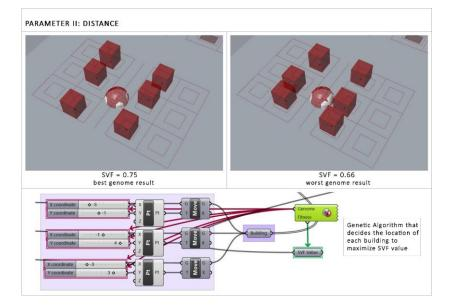
**Figure 9.** The SVF simulation based on the parameter, *distance*
