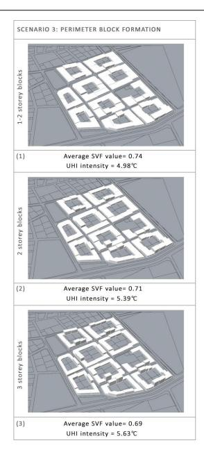
**Figure 17.** Compositional variations of the perimeter block typology, and the average SVF values of the fabrics generating a certain level of UHI intensity
