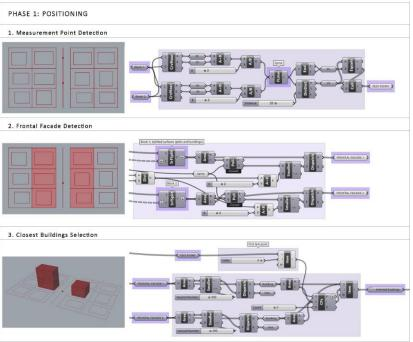
**Figure 5.** Phase 1: The consecutive steps to position the measurement point and the fields of analysis
