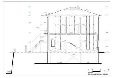
Figure 7: İbrahim Kaya Mansion B-B Section-Surveying Project (Karadayı Yenice, T., Dülgerler O.N., 2007)
