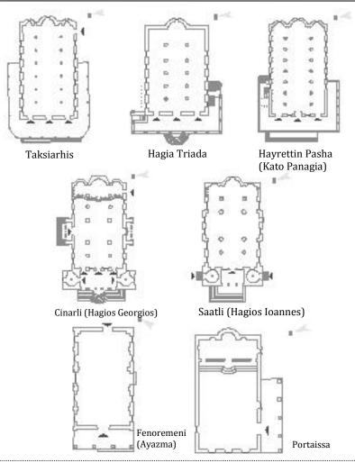
**Figure 2a.** Schematic plans of the church buildings that still exist in Ayvalik (İpek, 2003).
